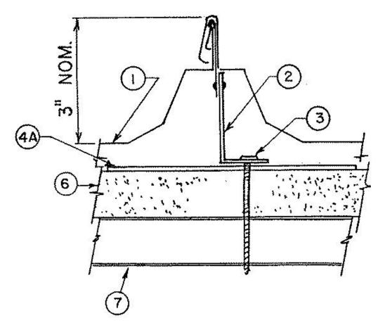
1. **Metal Roof Deck Panels\*** — No. 24 MSG min. Coated steel panels continuous over two or more spans. End laps to occur adjacent to purlins with panels overlapped 3 inch max. A line of sealant may be used at panel end and side laps.
